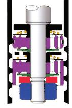
The PST design permits a wide range of tuning parameters. Almost any desired damping curve can be obtained while avoiding sudden transitions in performance between soft and hard damping modes. PST allows the choice of different damping forces for rebound and compression. This high degree of tuneability is of key importance to OEMs who desire specific ride characteristics.
