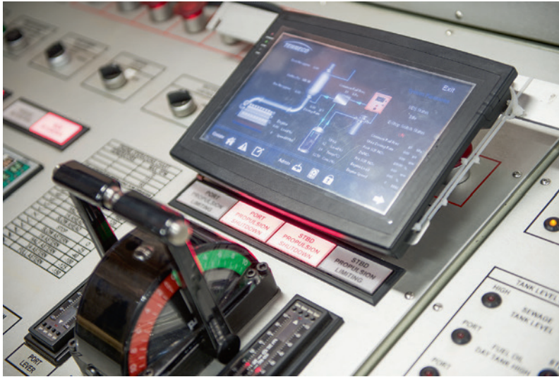
FIGURE 4 A 10" remote tablet HMI on the bridge of a ship (© Tenneco)
