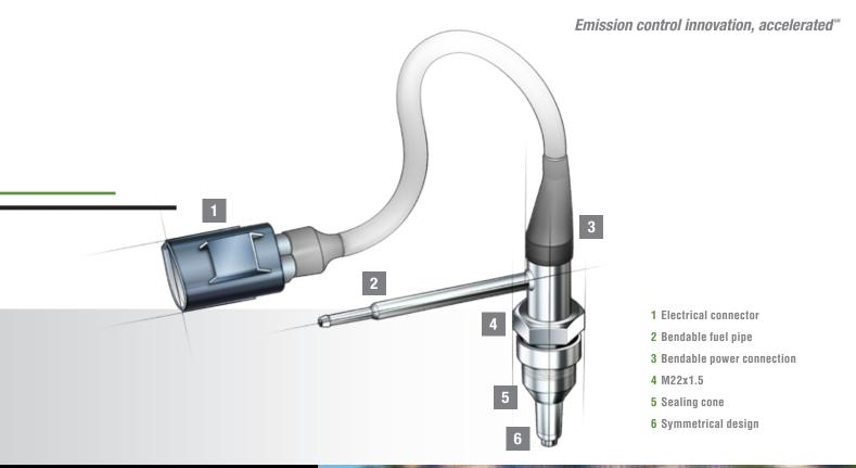
The Diesel Fuel Vaporizer is proven to avoid clogging and oil dilution, and reliably achieve full DPF regeneration.
