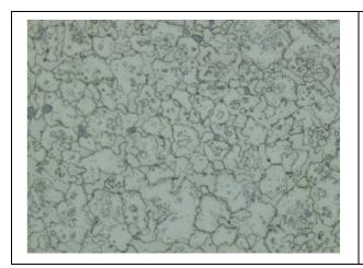
Micro structure (x500) of Tenneco's newly developed sintered steel material FM-T88A with 17 percent cobalt content
