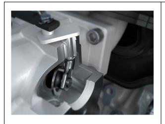
As a response to limited availability of cobalt and price volatility, Tenneco's Powertrain business group is developing wear-resistant materials with greatly reduced cobalt content. High temperature applications such as turbocharger wastegate shaft bushings and EGR valves are currently reliant on cobalt use to provide wear resistance in high temperature ranges and will benefit from the new materials.
